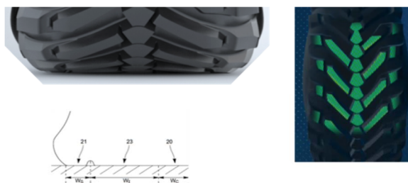
Fig. 4: Tire shape and contact patch in field configuration
