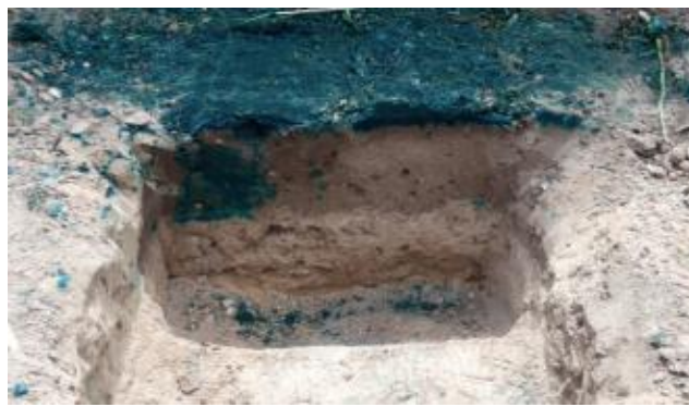
Results of infiltration tests with dye. On the left of the photo is a non-trafficked bed and to the right, an intermediate traffic lane.
