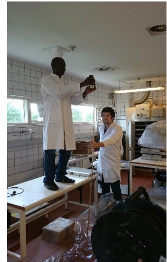
Fig. 5. Soil drop test on soil cores in the laboratory.
