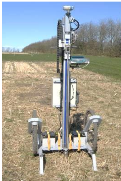
Fig. 5. Measuring soil penetration resistance using an automated cone penetrometer.
