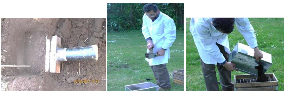
Fig. 3. Determination of aggregate size distribution (MWD) after a drop shatter test for soil taken from 10-20 cm depth.
